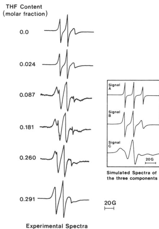
Figure 5. EPR spectra of TEMPO-labeled poly( N -isopropylacrylamide), PNIPAM-T/880, in water/tetrahydrofuran mixtures ( x_T : molar fraction of THF). Temperature: 20 °C. Polymer concentration: 4 g L -1 . Inset: simulated EPR signals of the three components A–C employed in the analysis of the EPR spectra of TEMPO-labeled poly( N -isopropylacrylamide).
